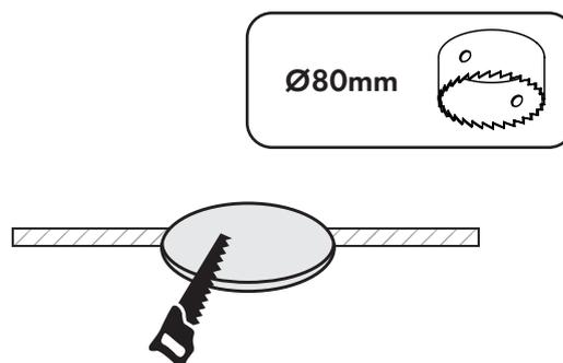
For new installations use suitable cutting tools and carefully cut the required hole.
