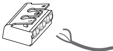
When wiring please ensure you have identified the correct wiring from the circuit and ensure the connections are tight and no loose strands have been left outside of the connection block.
