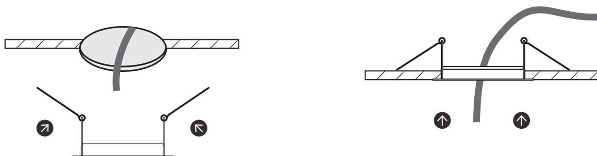
Push the springs upwards and fit into the ceiling hole ensuring the product is sitting properly and no cables are trapped.
