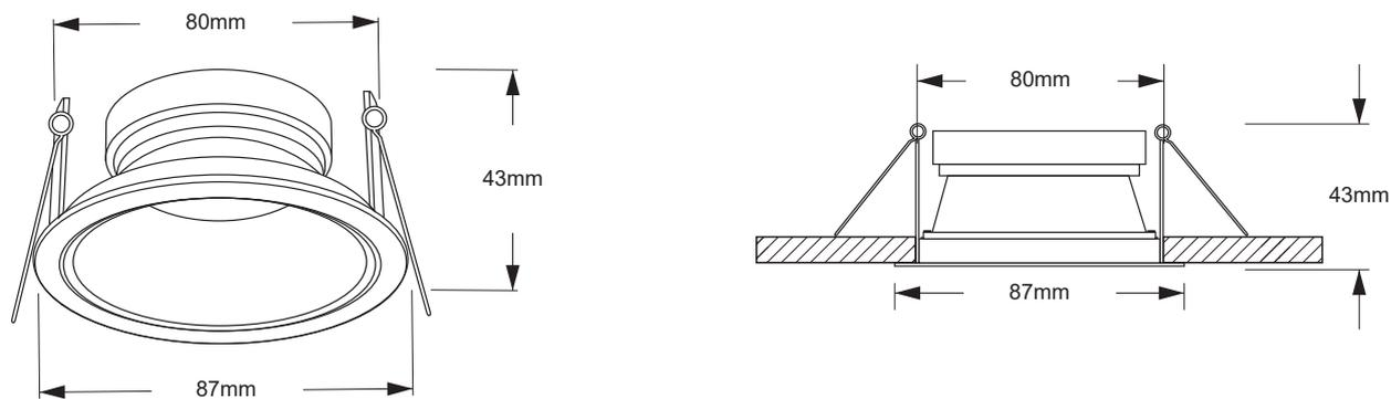
When installed in conjunction with our 'Insulation bracket' (Sold Separately) this product is suitable for coverage by thermal and acoustic insulation e.g. loft insulation. Not suitable for blown insulation. Please ensure a max wattage of 7W when covering with insulation and utilising the insulation bracket.
